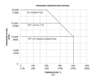
CAUTION: WHILE TESTING HAS SHOWN O-RINGS TO PROVIDE SATISFACTORY SERVICE LIFE, BOTH CYCLIC AND SHELF LIFE MAY VARY WIDELY WITH DIFFERING SERVICE CONDITIONS, PROPERTIES OF REACTANTS, PRESSURE AND TEMPERATURE CYCLING AND AGE OF THE O-RING. FREQUENT INSPECTION SHOULD BE MADE TO DETECT ANY DETERIORATION AND O-RINGS REPLACED AS REQUIRED.
