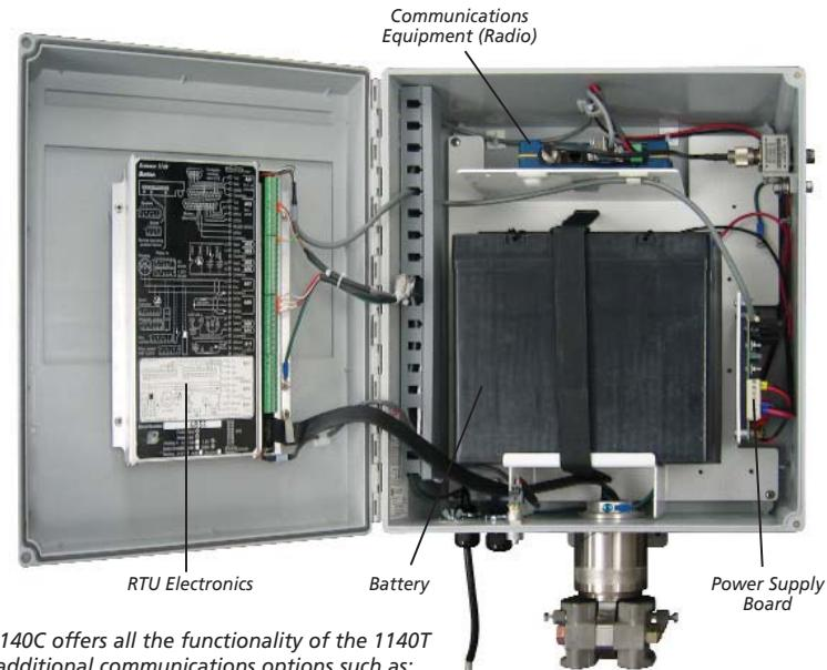
*The 1140C offers all the functionality of the 1140T with additional communications options such as: integral radio, cellular modem, and dial-up modem capabilities.*
