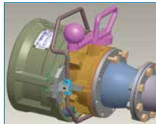
Align coupler bolt holes with bolt holes on loading device.
