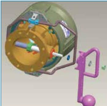
Install the new load distribution washer on the handle shaft with the permanent mark toward the assembler. Install the operating handle, the new lock washer, and new 10 mm nut. Tighten the 10 mm nut using the 11/16-inch or 17 mm deep reach socket to 25 ft-lb, or 34 N•m torque.
