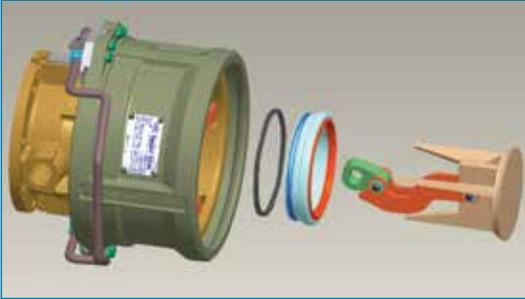
Remove the poppet assembly, cylinder, and cylinder wave spring.
