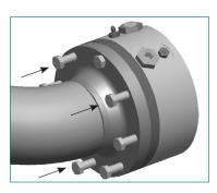
**Step 4:** With the rest of the loading arm still secured from movement, loosen the bolts on the other side of the swivel. Swivel module should fall away easily to expose environmental and O-ring seals. Secure product seal.
