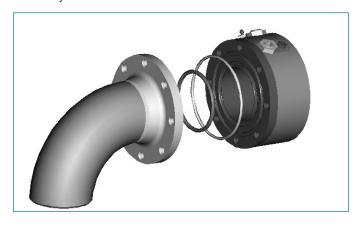
**Step 4:** Carefully remove dynamic environmental seal. Clean and inspect all machined surfaces and carefully press new environmental seal into groove. NOTE: Lube seal with light machine oil.
