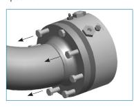
Step 6: Align flange with body and press surfaces together. Thread flange bolts with Nord-Lok™ washers into tail and torque to amount shown on chart. Nord-Lok™ washers come as an assembly bonded together from the factory. It is important that the correct
