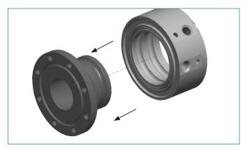
**Step 3:** After all balls have been removed, carefully remove swivel tail from swivel body.
