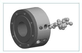
**Step 6:** Install ball bearings until bearing chamber is full. Chart below shows the number of bearings per race.
