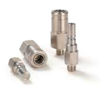
The RNS are rigid couplings with flat face valves. They can be mounted on rigid manifolds or tubing and assure connection/disconnection without spillage. Base material is brass and stainless steel.
