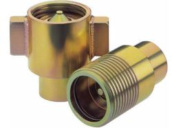
and Gas Industry. This third-party certification (Lloyd's Register Certificate NAO 0701023/1) verifies that this product meets the standards of API 16D and the Alberta Energy and Utilities Board - EUB Directive #36. These units were tested at 700°C (1300°F) fire exposure for 5 minutes at full operating pressure without loss of pressure or leakage.
