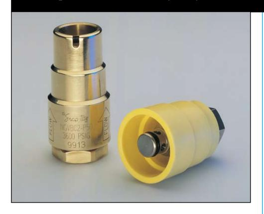
Snap-tite's inline breakaway is designed specifically for compressed natural gas fueling systems. When properly installed, this inline breakaway allows for the safe disconnection from the fueling system without damage to the dispenser in the event of an accidental disconnect (drive-off). The inline breakaway was designed to replace the traditional tripod leverage towers used in conjunction with the ISO B style coupling as the breakaway connection for the fueling hose from the dispenser.
