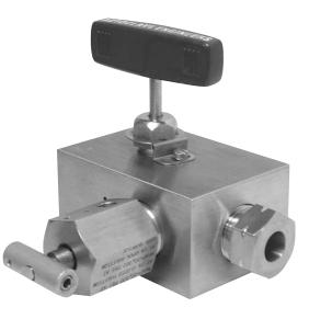
Autoclave's Wellhead Gauge valves are designed for reliable shut-off service at a maximum working pressure of 30,000 psi (2068 bar). The Wellhead Gauge and Bleed Valves are standard in 316 stainless steel material. Special materials available on request.
